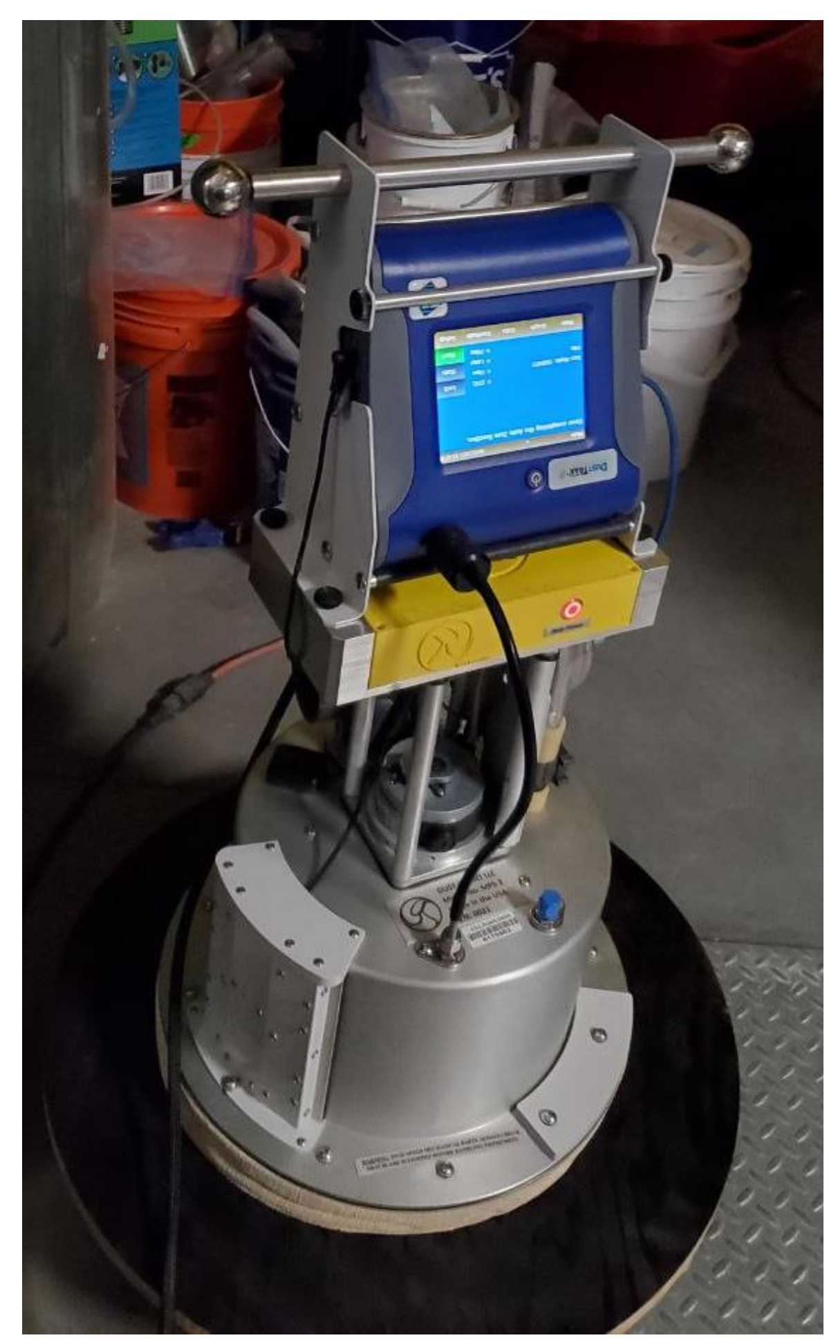
Running Pi-SWERL in the pan specimens in the lab
