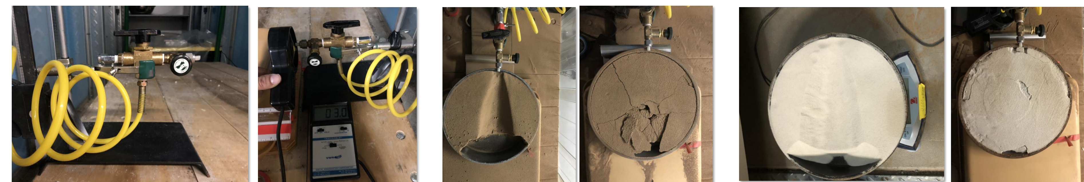
Wind erosion testing of untreated and EICP treated soil pans with the air jet setup.
