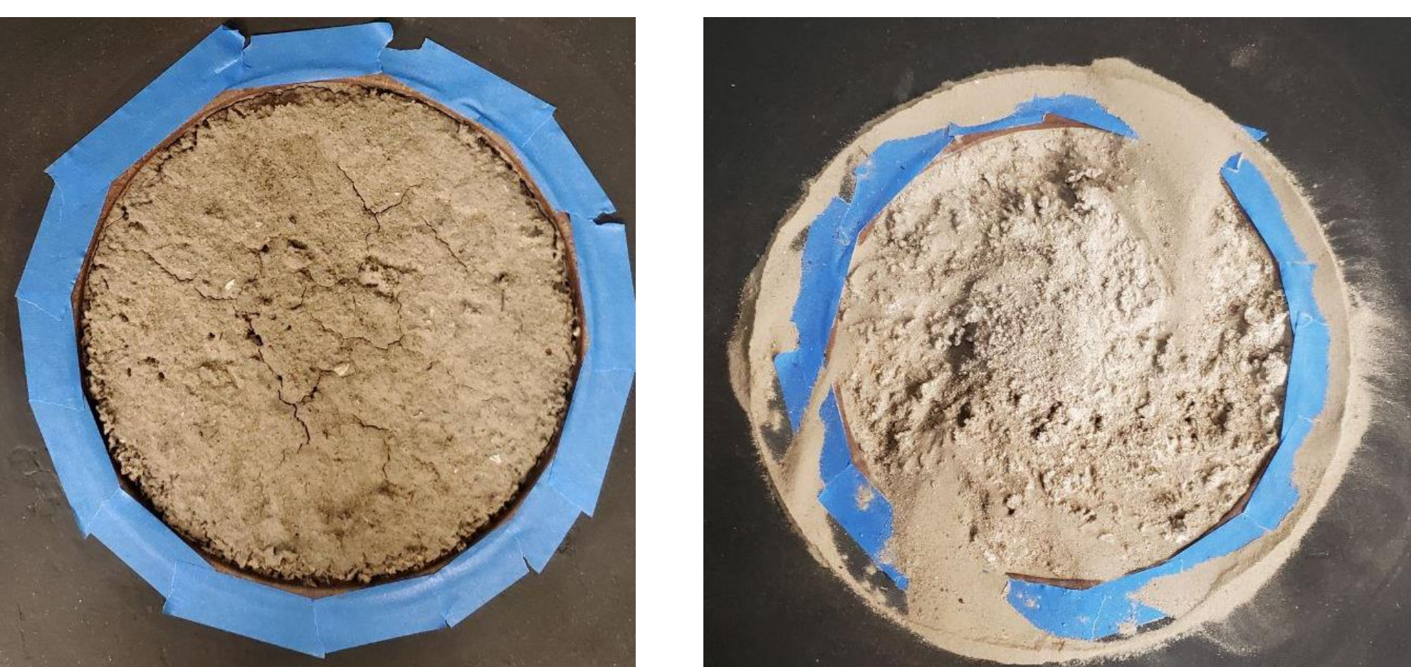
Treated (using MICP 0.5 M urea + CaCl2) vs. untreated sample after testing with PI-SWERL
