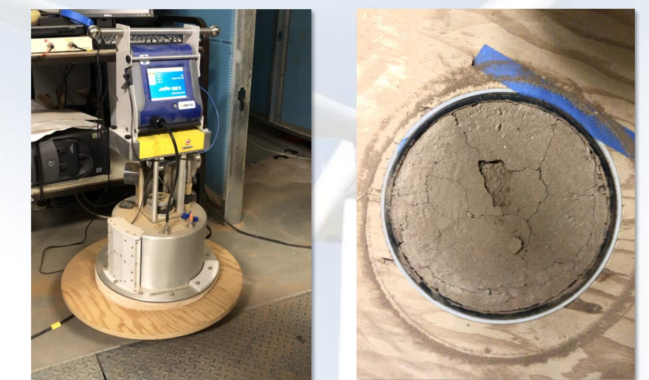
PI-SWERL test of an EICP treated soil pan.
