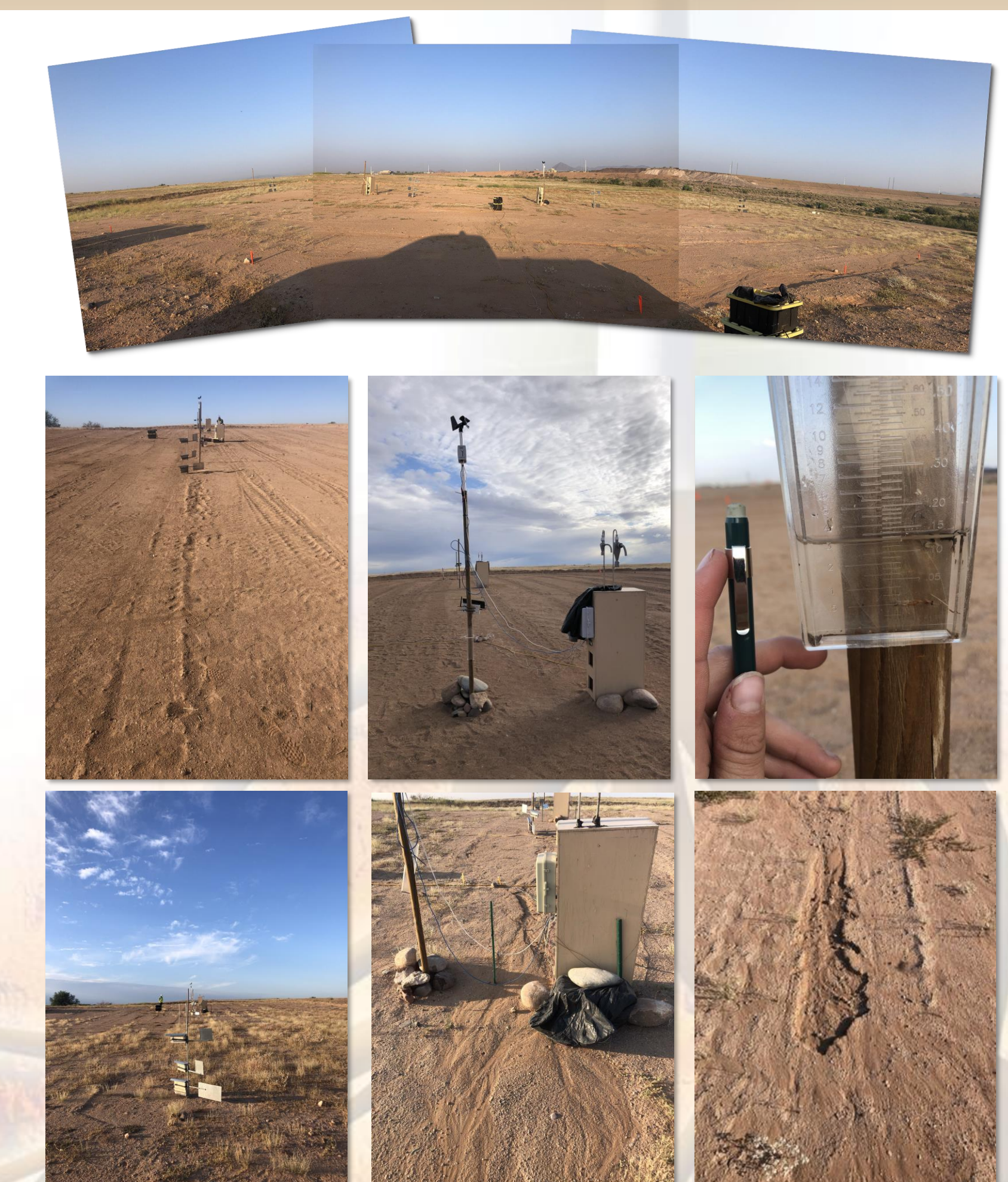
Measurement of background site conditions including wind speed/direction, dust emissivity, and carbonate content.
