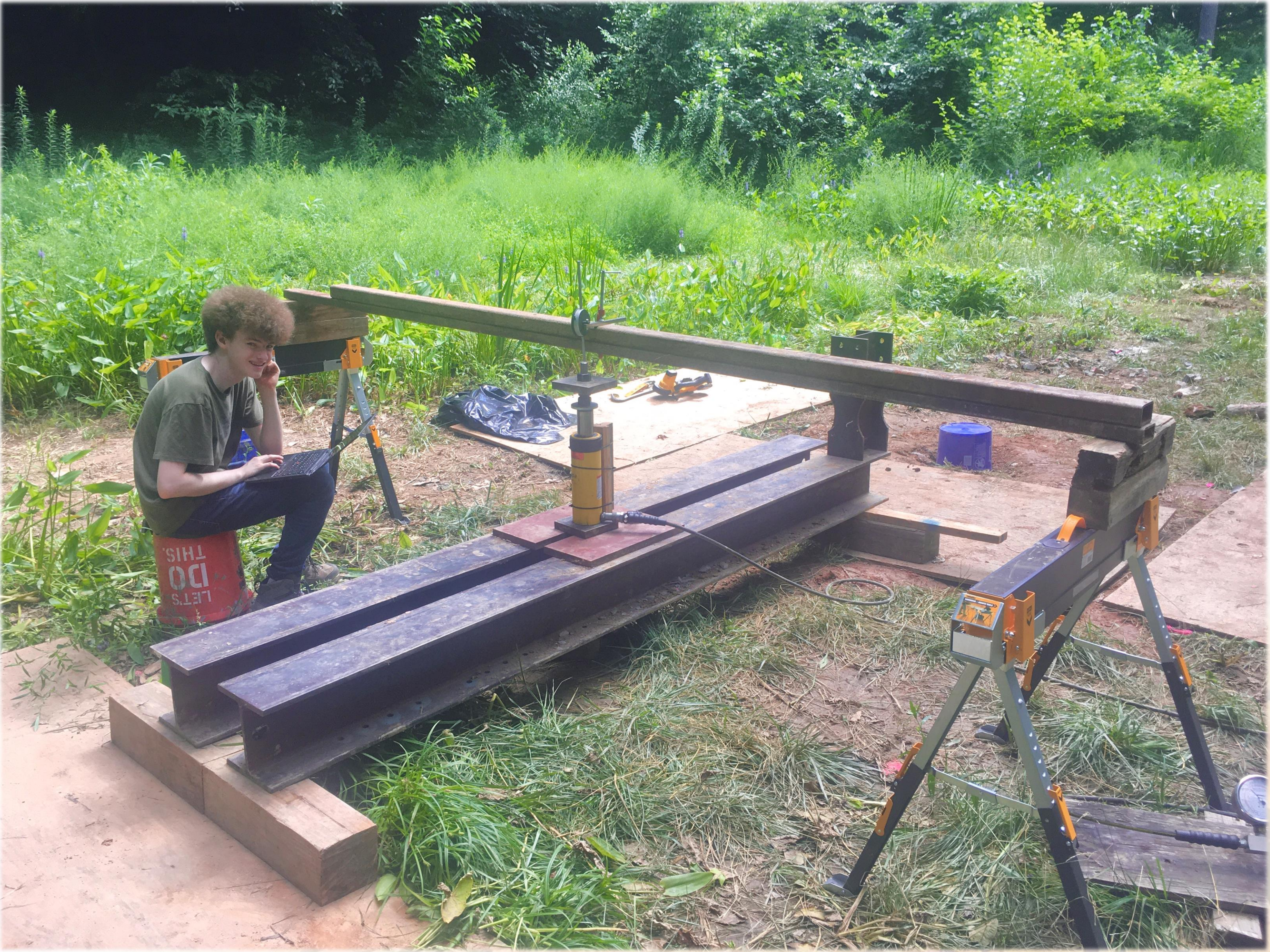
A Young Scholar collects data during pullout load testing – June 2021
