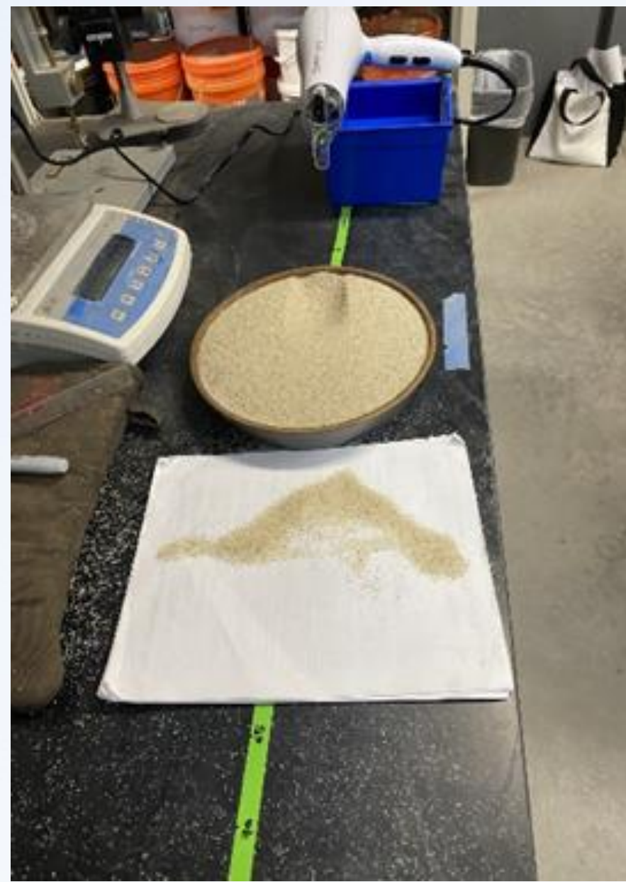
Untreated soil wind erosion test
