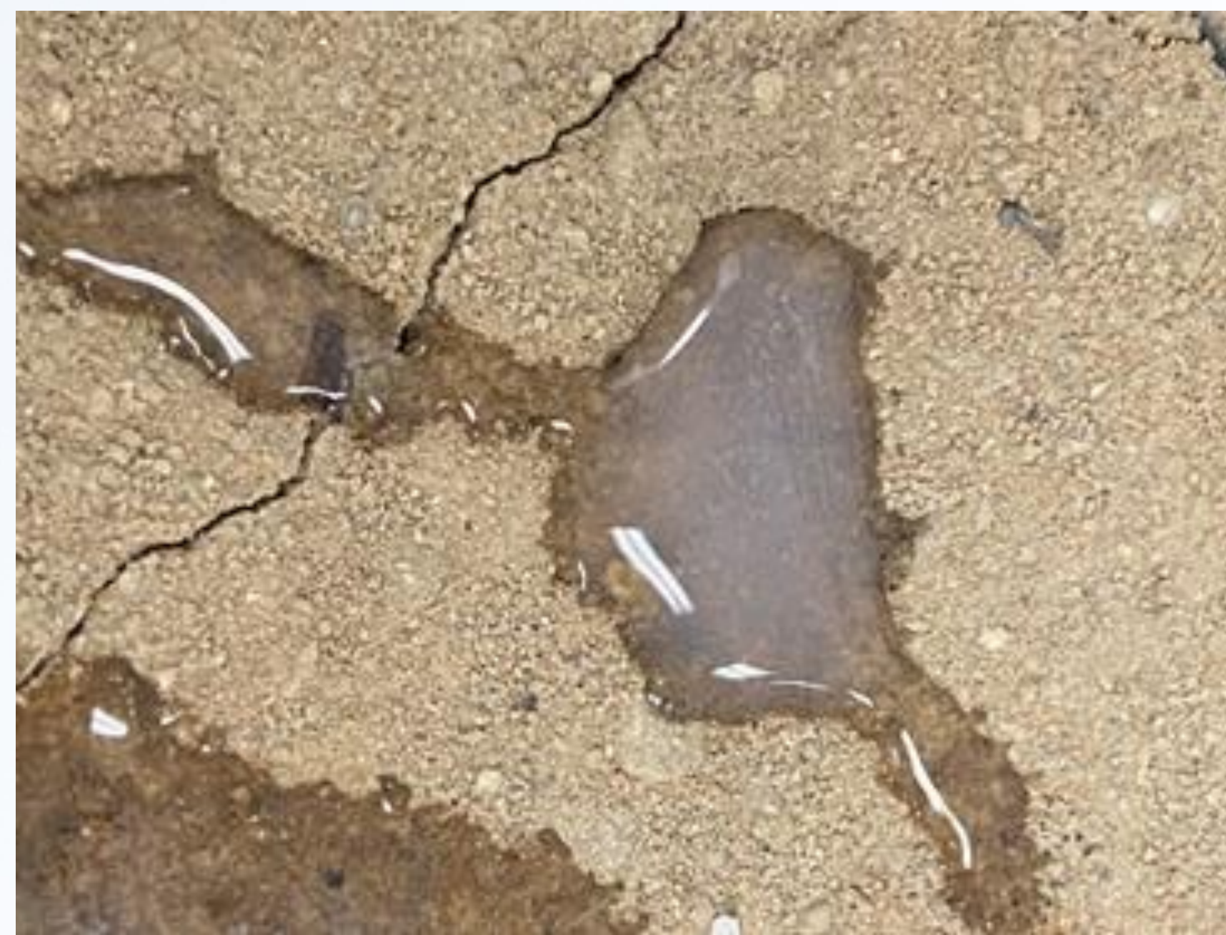
EICP treatment soaking in the soil
