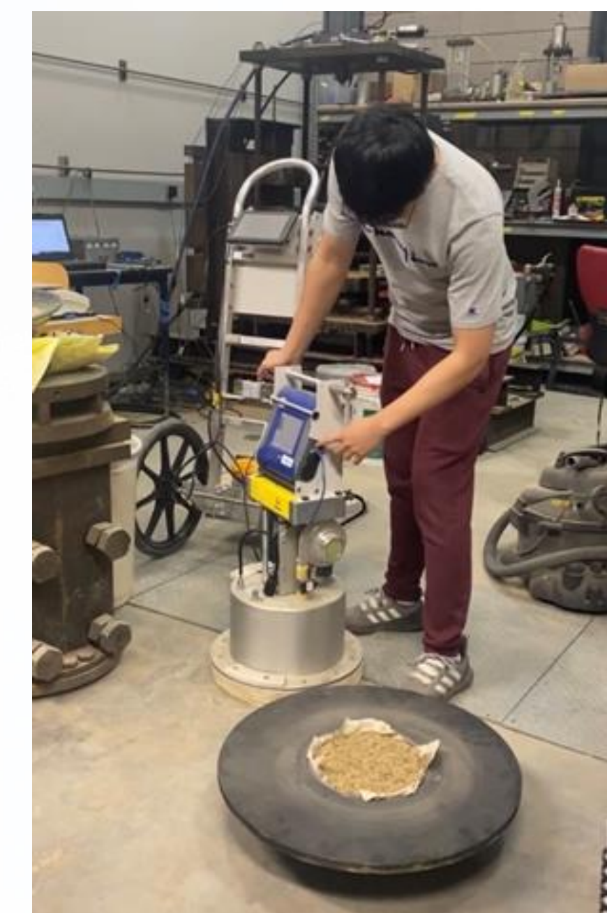
Xi Yu performing P-Swirl test on untreated soil
