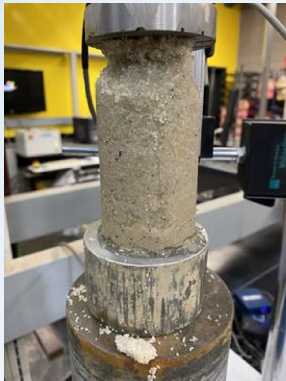
EICP column compression test
