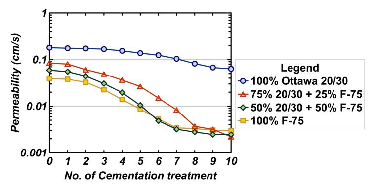
The obtained results from MICP experiments are shown in the figure above.
